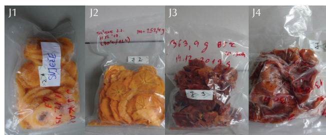
Fig. 1 – Samples of fresh and dried Japanese persimmon: (J1) fresh Japanese persimmon (control sample); (J2) drying at 70 °C/12 h; (J3) drying at 85 °C/10.5 h; (J4) drying at 100 °C/5.5 h
