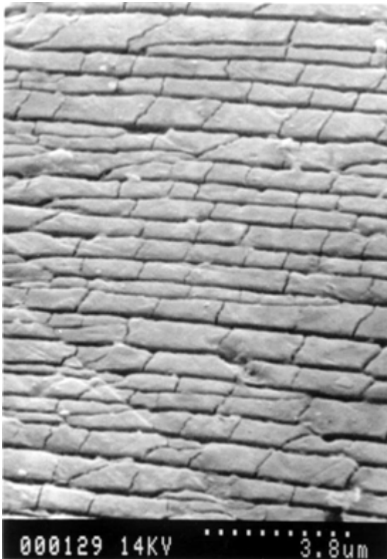
Fig. 6C – SEM image of a thin gel layer deposited on such an irregular surface
