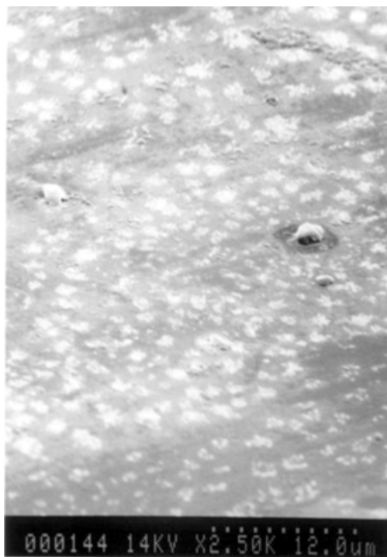
Fig. 5 A – SEM image of a translucent layer with well developed micro-crystals of anatase (873 K)
