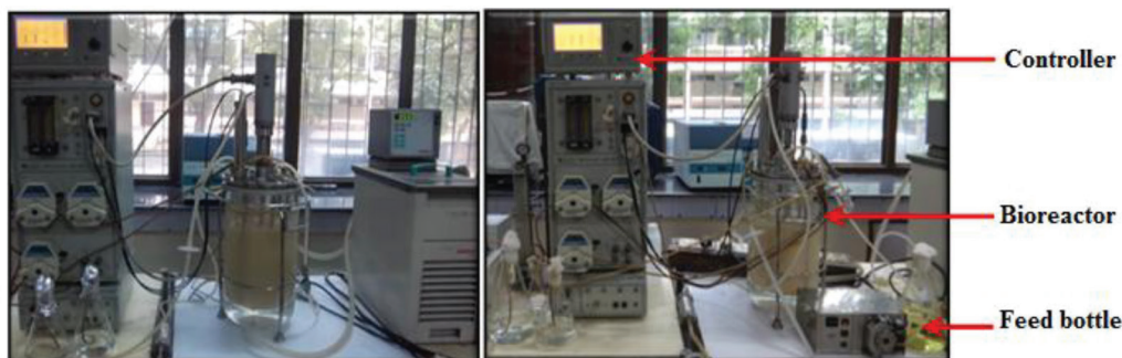
Fig. 1 – Complete experimental set up of (a) batch cultivation (b) repeated-batch cultivation in the 7-L bioreactor (Applikon Dependable Instrument, The Netherlands)
