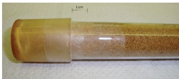
Fig. 2 – Racing tubes showing solid-state cultivation on beech sawdust substrate. Mycelial growth is visible with the naked eye.
