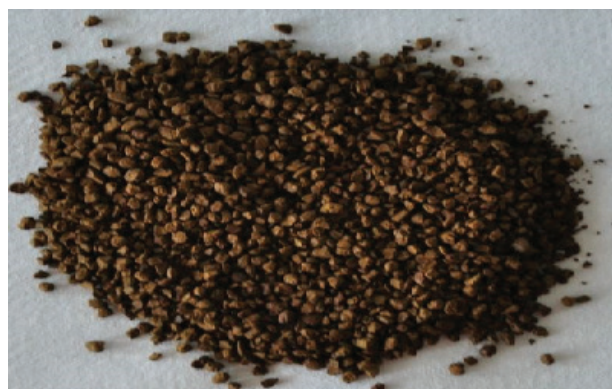
Fig. 1 – Granular ferric oxide 29
